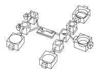
This is a PCR microfluidic system connected by multiple modules.
