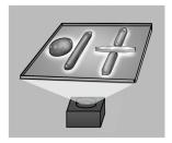
Light patterns are used to elongate the droplet and move it across the surface. The droplet is sliced with an integrated Teflon blade on the light-actuated digital microfluidic platform. Droplets are manipulated using different temperatures on the surface.
