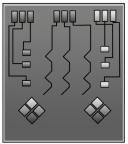
A portable whole-cell biochip used to monitor water geno-toxicity. The chip is controlled using external electric fields. A microfluidic device that uses charged electrodes to control the motion and mixing of droplets.
