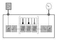
The temperature can be controlled within this microlfuidic device through the applied voltage.
