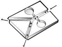
A particle-sorting module that helps to filter the cells of interest from the sample.
