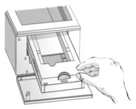
This device reads fluorescent signals from a microfluidic assay that has already completed its reaction(s). Two independent microfluidic systems are connected together through the mixing chamber.
