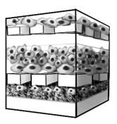
This organ-on-chip device makes use of both surfaces for culturing different types of cells. These PDMS microchannels incorporate a porous membrane in between the culture cells.
